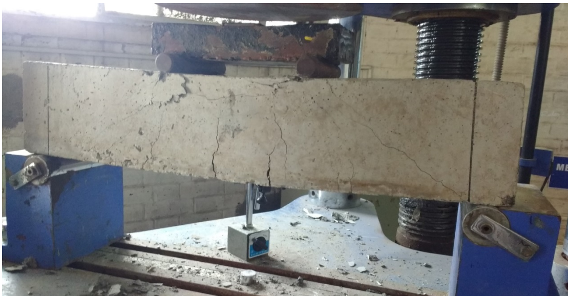
Fig 5.7 Shear - Flexure failure of beam
