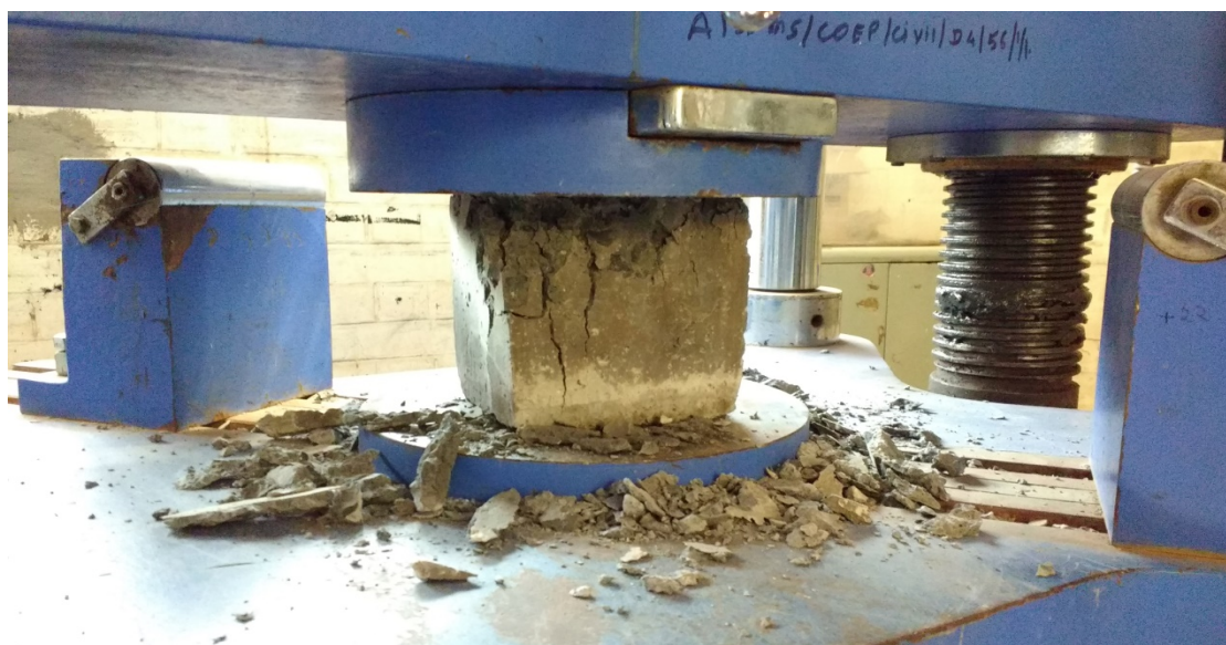
Fig 5.1 Testing of cube
